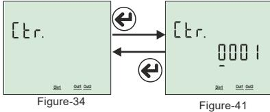
To change the current transformer ratio, press the set button while the figure-34 is on the screen. Figure-41 comes to the screen. Press right button to move between digits. Press the down key to change the value of the digit. You can change the digit value which is the underline. When you press the set button after entering the ratio, the current transformer ratio is recorded and the screen shows figure-34. You can scroll through the parameters
