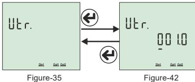
To change the voltage transformer ratio, press the set button while the figure-35 is on the screen. Figure-42 comes to the screen. Press right button to move between digits. Press the down key to change the value of the digit. You can change the digit value which is the underline. When you press the set button after entering the ratio, the voltage transformer ratio is recorded and the screen shows figure-35. You can scroll through the parameters
