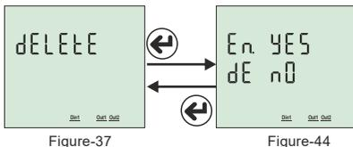
To delete the records, press the set key while figure-37 is on the screen. Figure-44 comes to the screen. You can delete 2 records here. Energy (En) and Demand (dE). Press the right key to move the point (.) to the record which you want to delete. Then press the down key to change the value to "yes". The record value which you do not want to delete must remain in "no".
