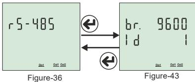
To change the RS-485 remote communication settings, press the set button while figure-36 is on the screen. Figure-43 comes to the screen. Two parameters can be set here. Baudrate (br - communication speed) and Modbus ID (id - the number that identifies the device on the RS485 line). Press the right button to move the point (.) to the parameter you want to set.
